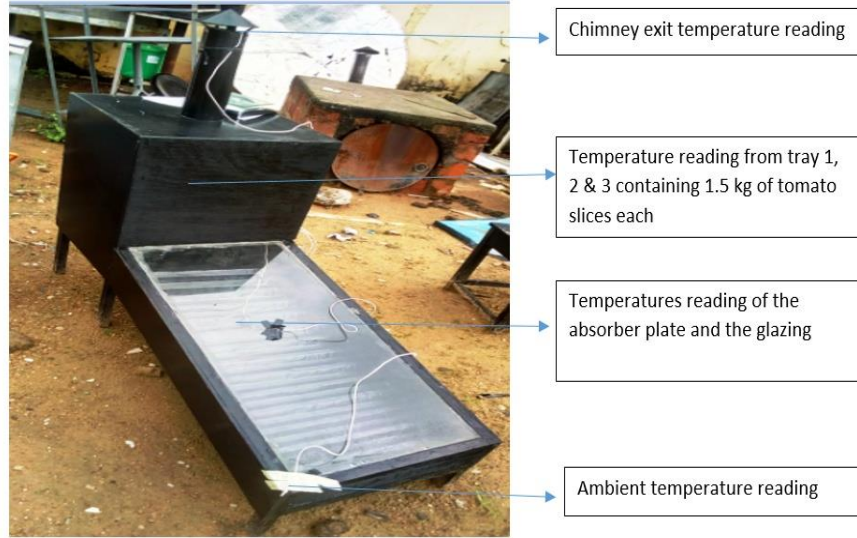
Figure 5: Experimental set up of the solar drying
